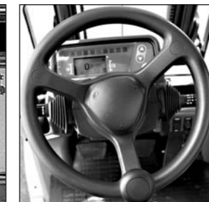
Fully hydrostatic steering
